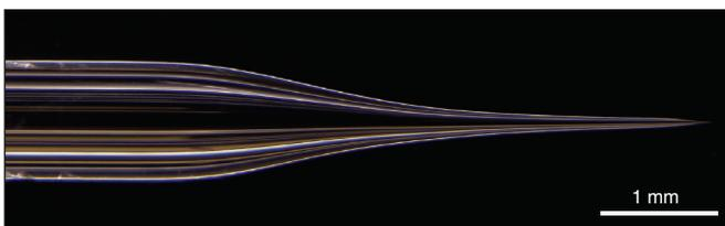
**FIGURE 1.** Overview of an injection needle. Note that the tip of the needle can be broken by gently rubbing it on a Kimwipe.
